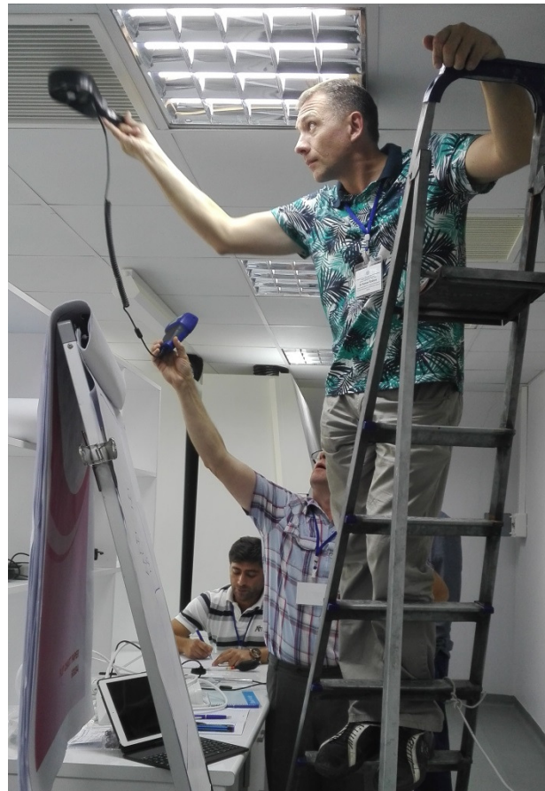
Fig. 4. A training participant uses a vane anemometer to measure the upper-room ventilation system airflow.
