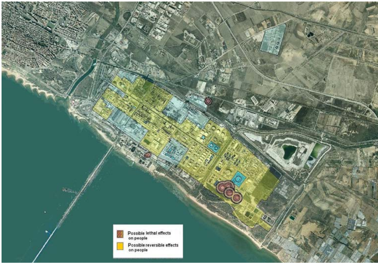
Fig. 36. Fire of flammable substances
