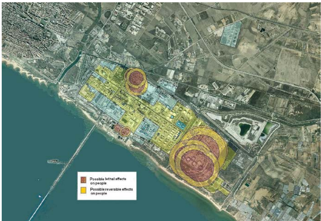
Fig. 35. Flash fires of flammable and highly flammable substances and liquefied petroleum gas
