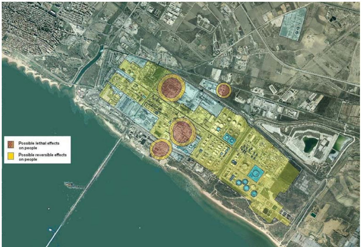
Fig. 38. Flash fire of liquefied petroleum gas
