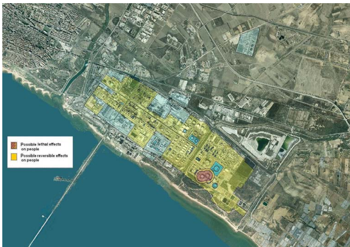
Fig. 39. Dispersion of flammable substances
