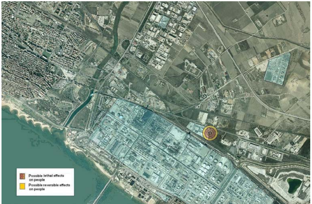
Fig. 37. Flash fire of highly flammable substances
