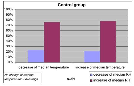
In the control group, there is always an increase of humidity irrespective of whether the indoor temperature goes up or down. In the intervention group, a decrease of indoor temperature in comparison to the year before the intervention does not have any effect on humidity levels, while an increase of humidity is observed in dwellings with higher temperature than in the year before.
